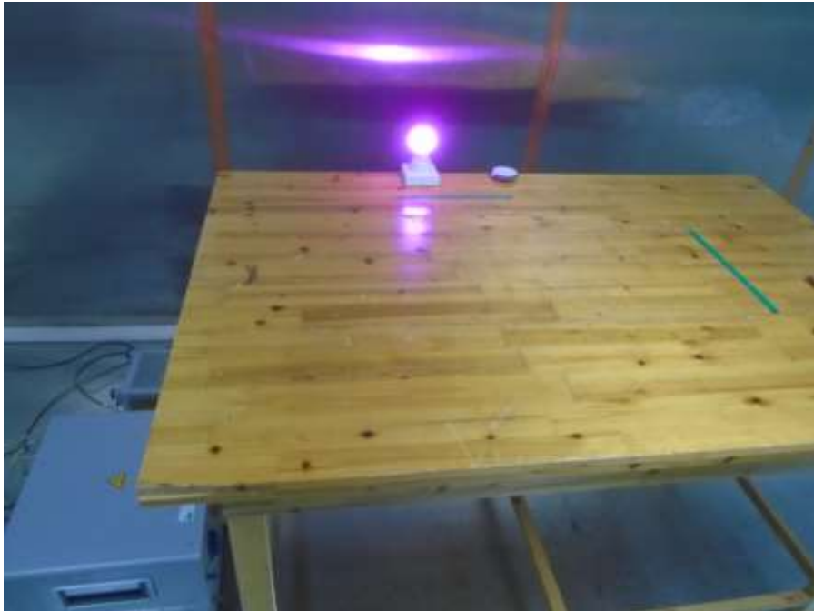
Photograph 1: Set-up for measurement of conducted emission
