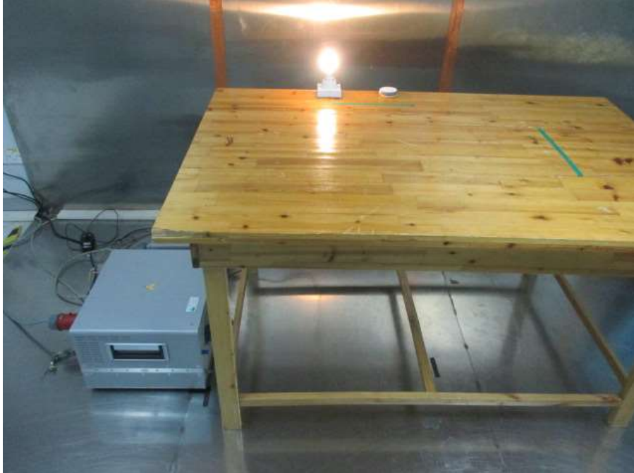
Photograph 1: Set-up for measurement of conducted emission
