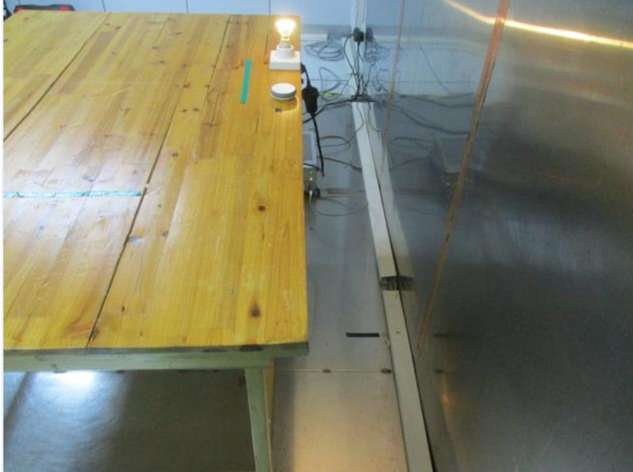
Photograph 1: Set-up for measurement of conducted emission
