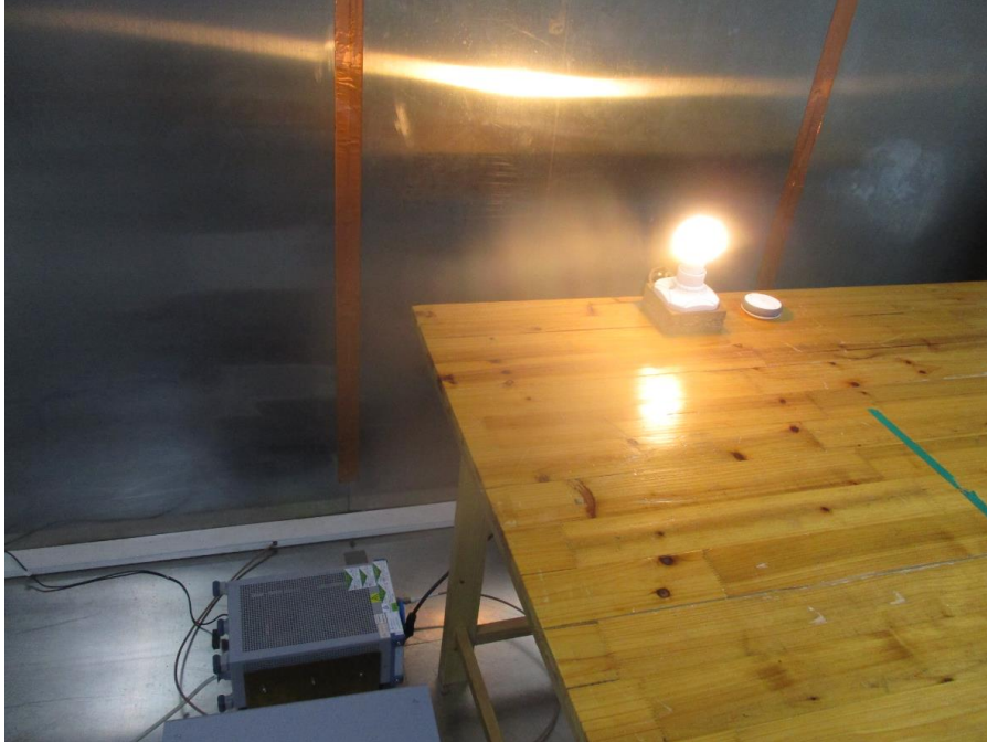
Photograph 2: Set-up for measurement of radiated emission
