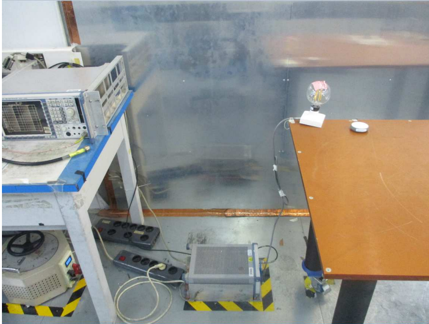
Photograph 2: Set-up for measurement of radiated emission
