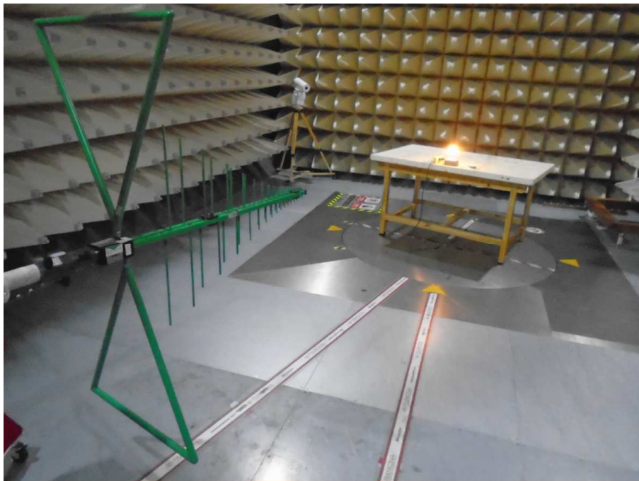
Photograph 2: Set-up for measurement of radiated emission
