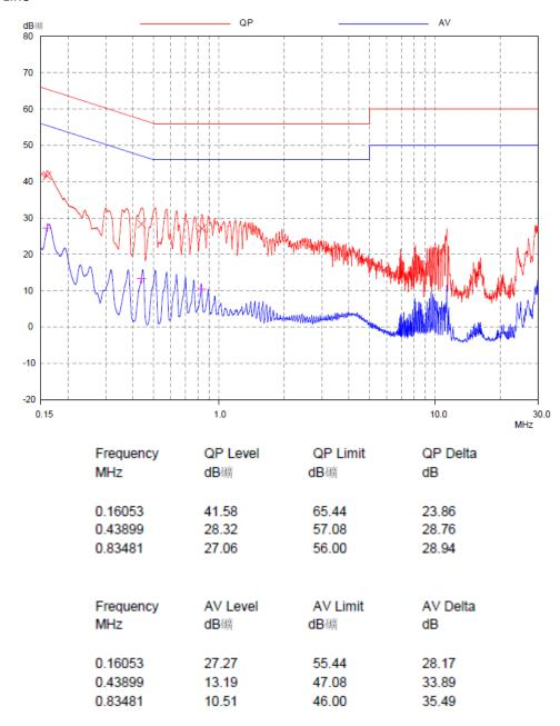
Remark: 1. Correct Factor = LISN Factor + Cable Loss, the value was added to Original Receiver Reading by the software automatically.
