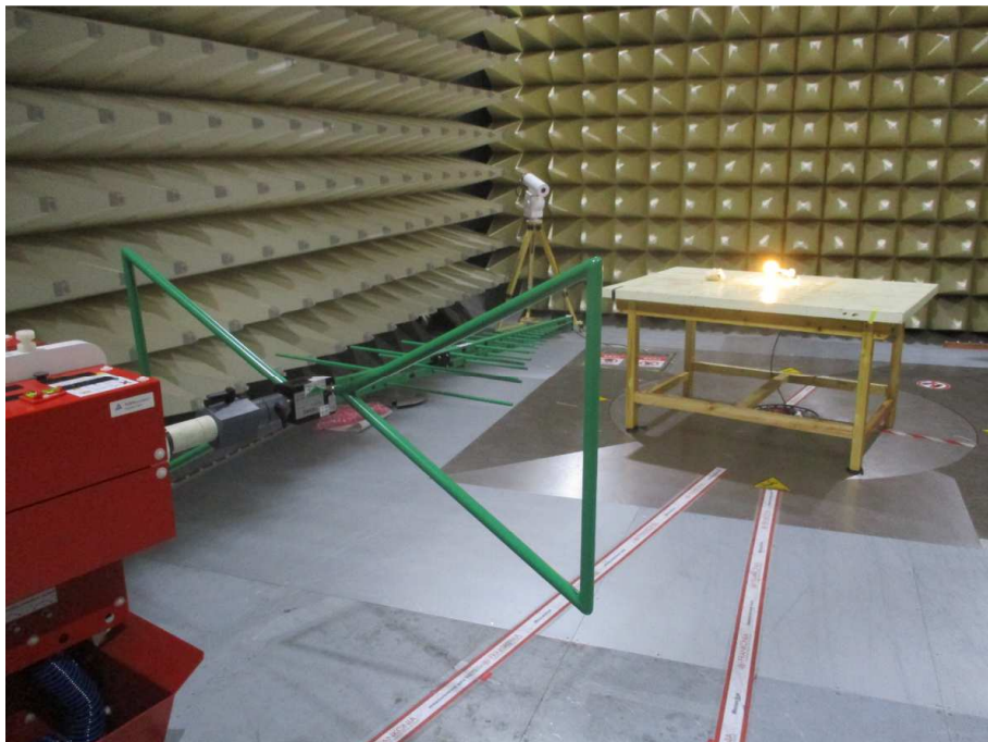
Photograph 2: Set-up for measurement of radiated emission
