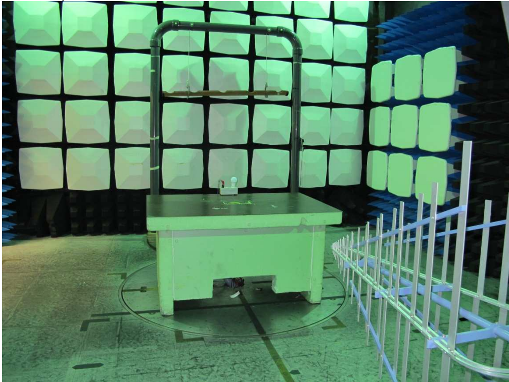
Test set up radiated emission 1GHz – 18 GHz
