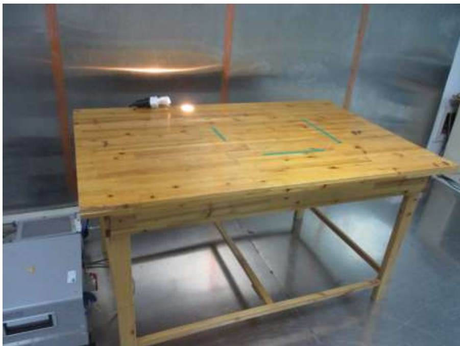
Photograph 1: Set-up for measurement of conducted emission
