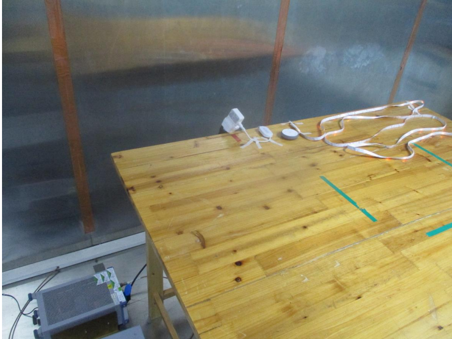
Photograph 1: Set-up for measurement of conducted emission
