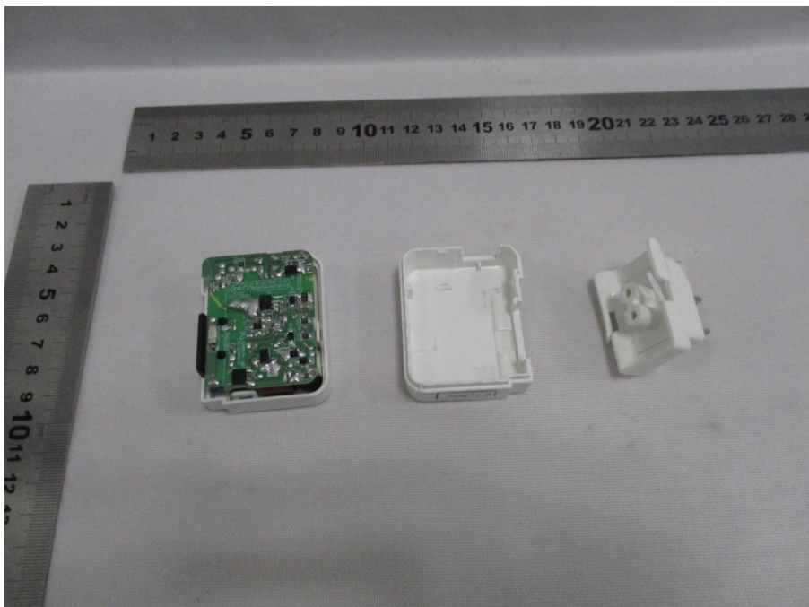
Open view of power supply
