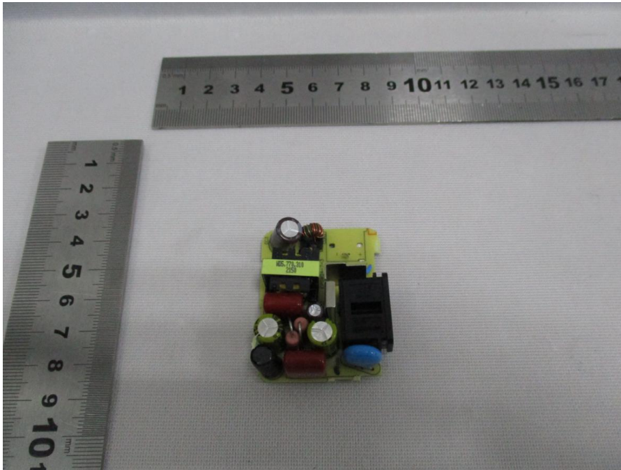
PCB of power supply
