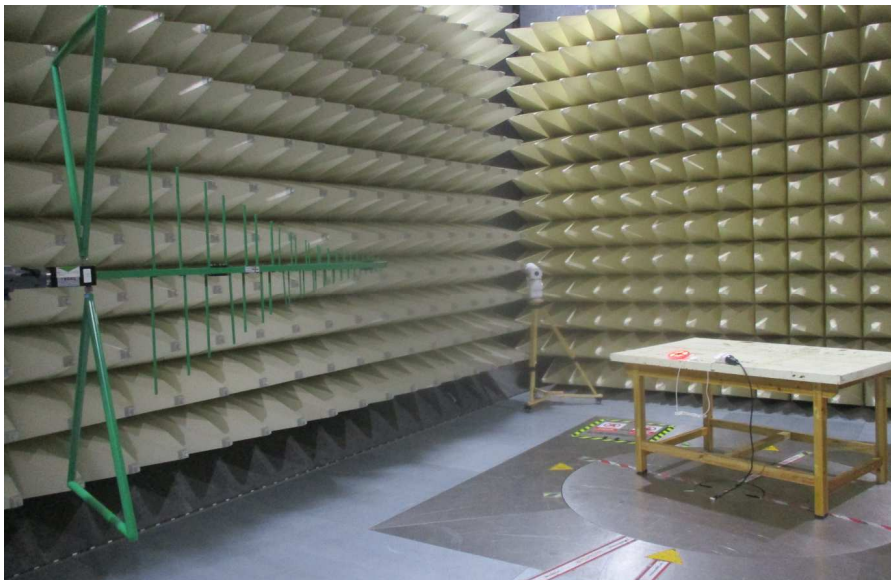
Photograph 2: Set-up for measurement of radiated emission
