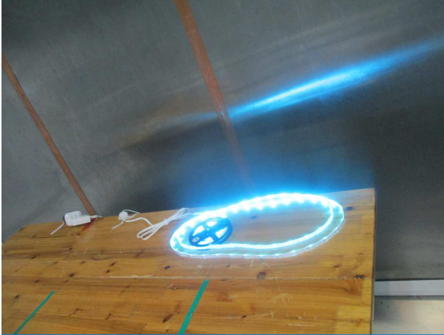
Photograph 1: Set-up for measurement of conducted emission
