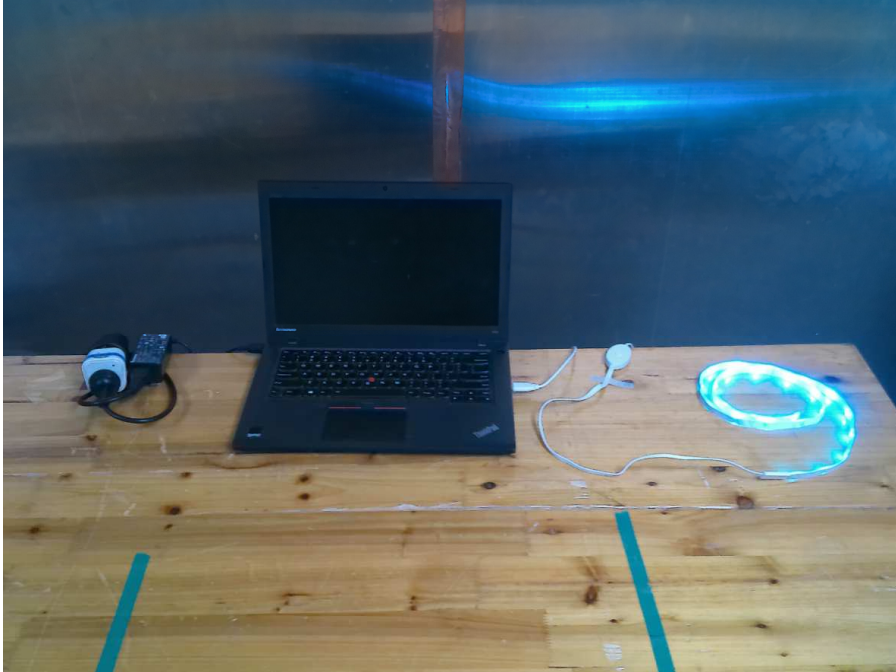
Photograph 1: Set-up for measurement of conducted emission
