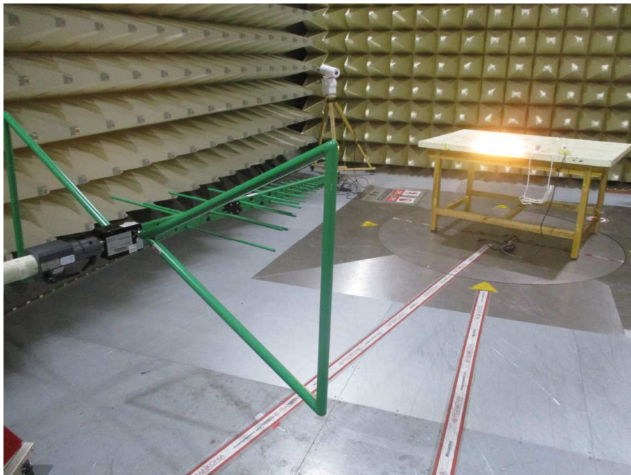
Photograph 2: Set-up for measurement of radiated emission
