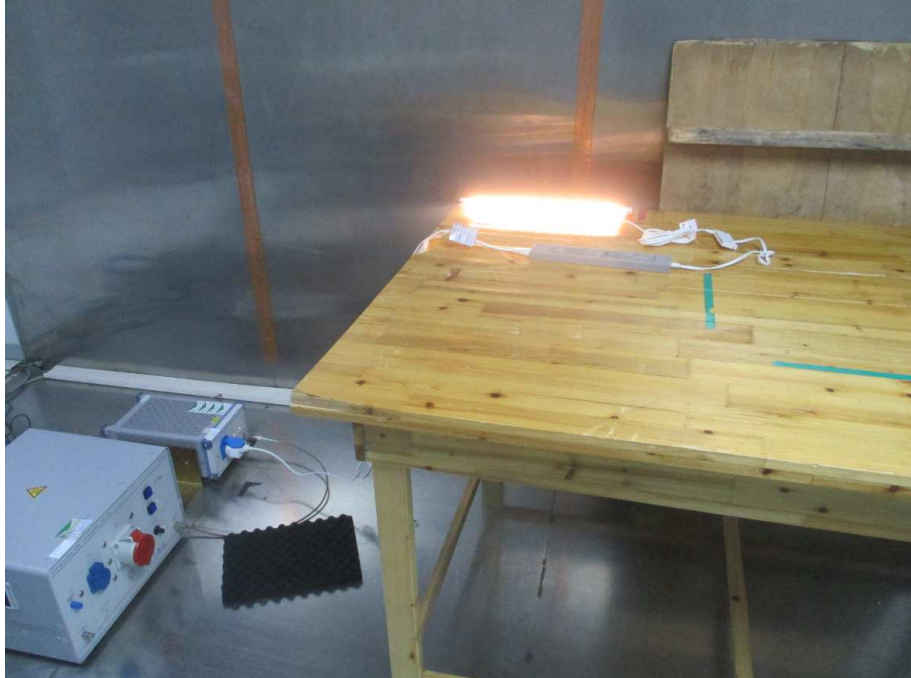
Photograph 1: Set-up for measurement of conducted emission
