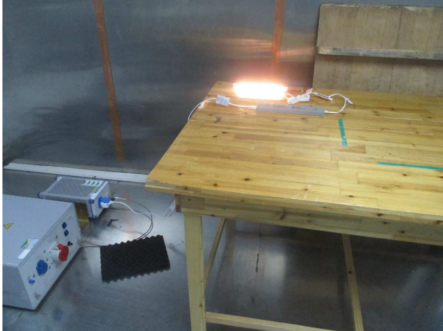
Photograph 1: Set-up for measurement of conducted emission
