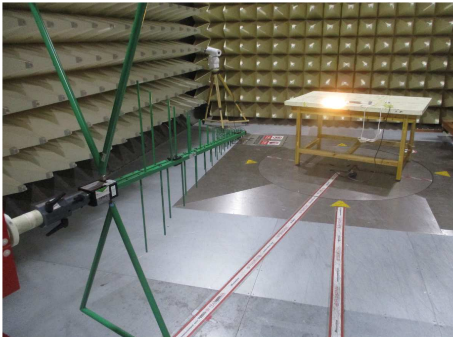
Photograph 2: Set-up for measurement of radiated emission
