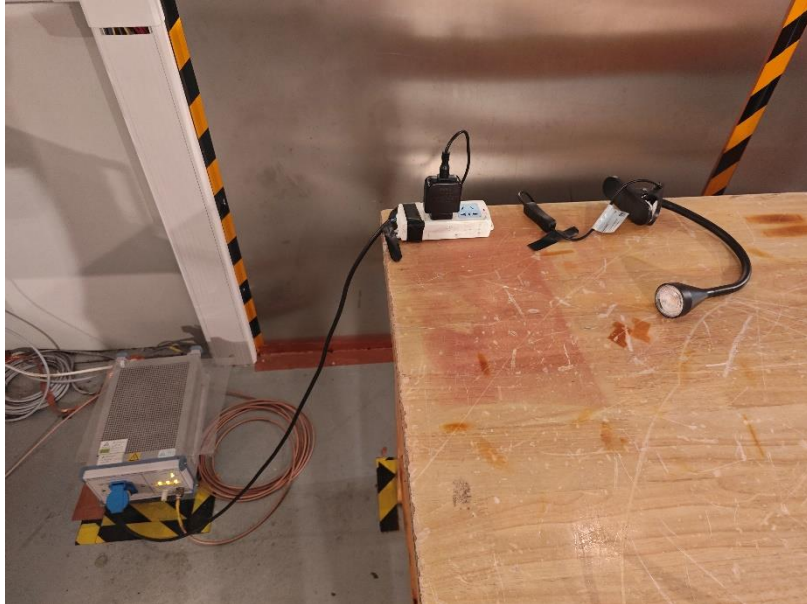
Photograph 1: Set-up for measurement of conducted emission
