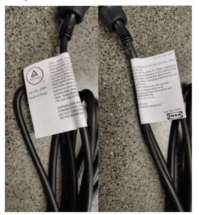
The Power line is undetachable part of the Portable general purpose luminaires.
