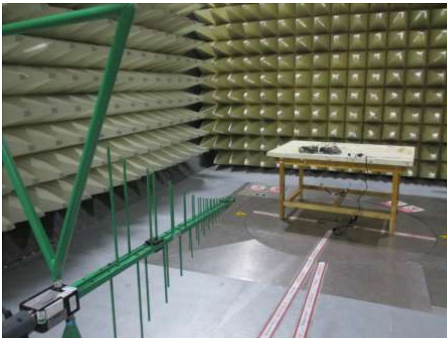
Photograph 2: Set-up for measurement of radiated emission
