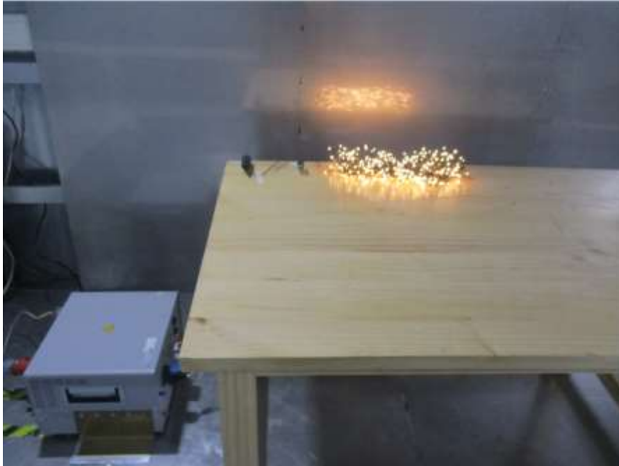
Photograph 2: Set-up for measurement of radiated emission
