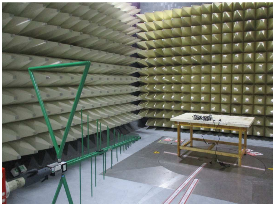
Photograph 2: Set-up for measurement of radiated emission
