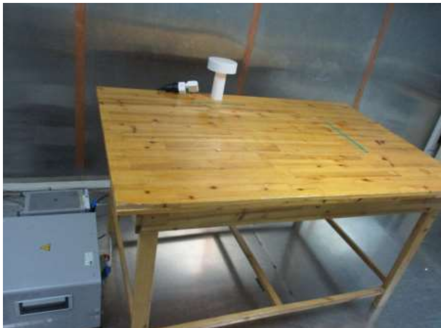
Photograph 1: Set-up for measurement of conducted emission
