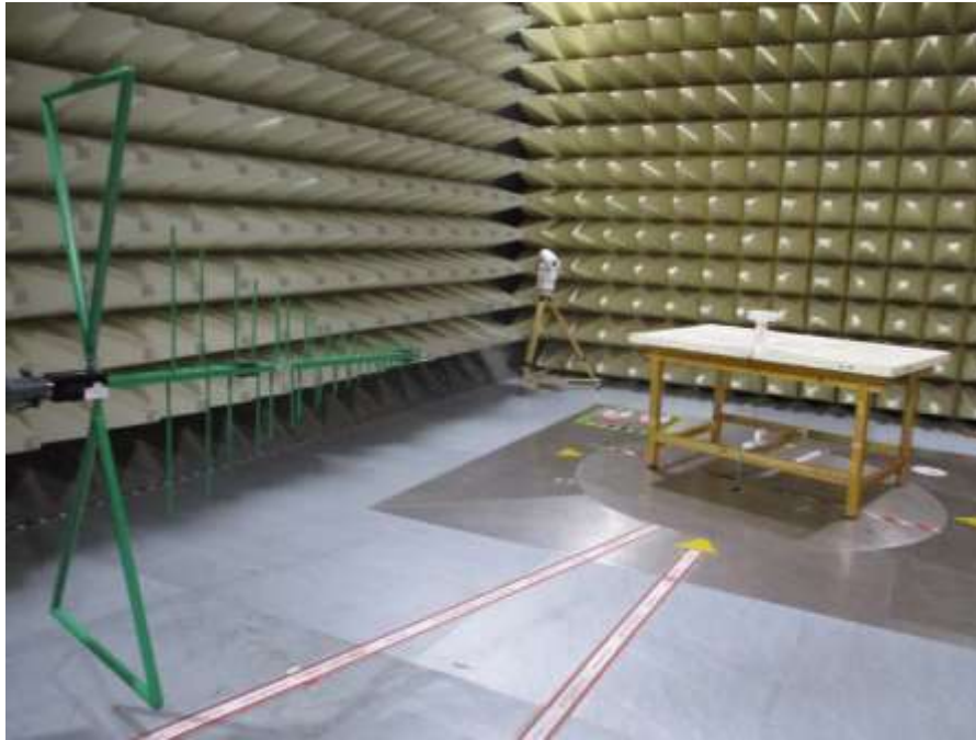
Photograph 2: Set-up for measurement of radiated emission
