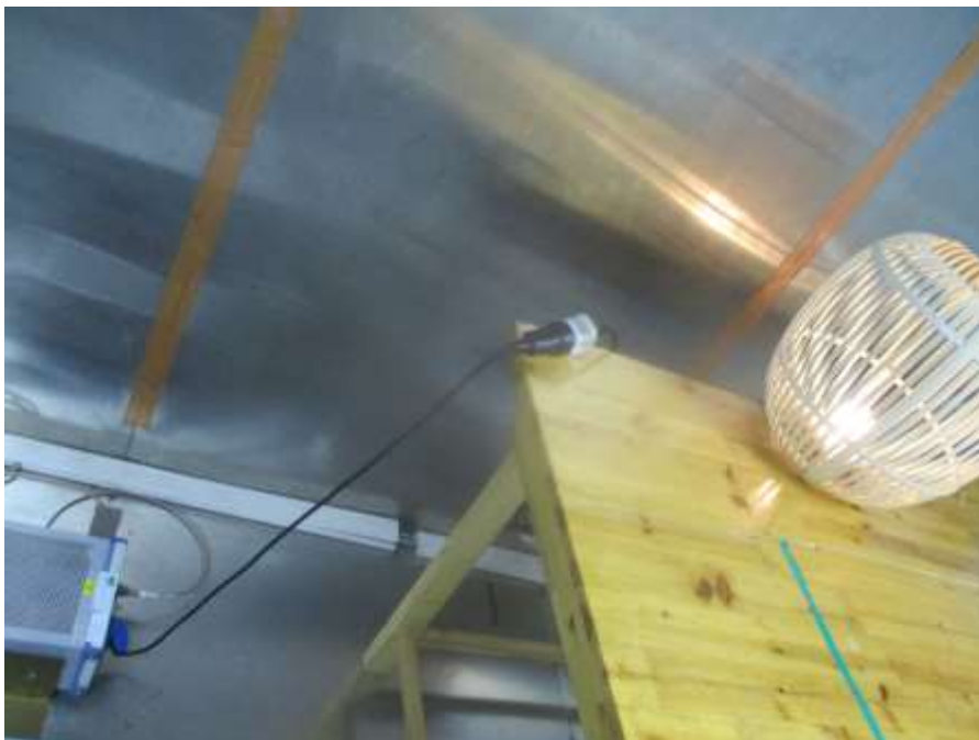
Photograph 1: Set-up for measurement of conducted emission
