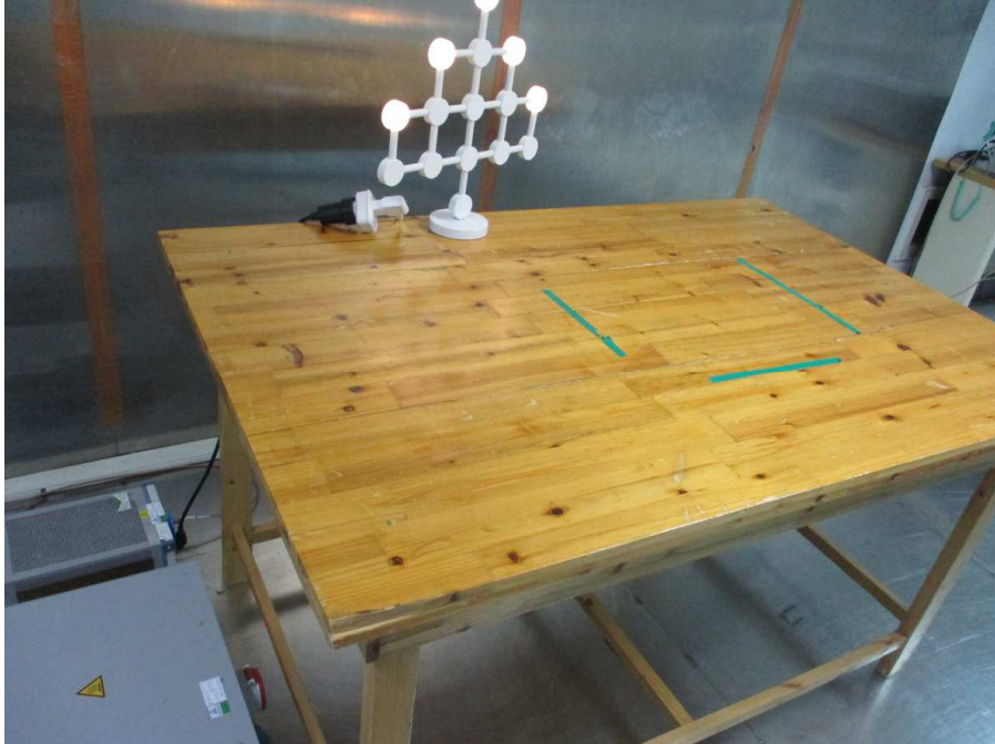
Photograph 1: Set-up for measurement of conducted emission
