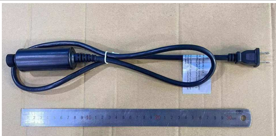
External view of power unit
