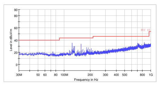
The emission levels with 960 to 1000 MHz also comply with the ICES-005 limit 46 dB $\mu$ V/m.
