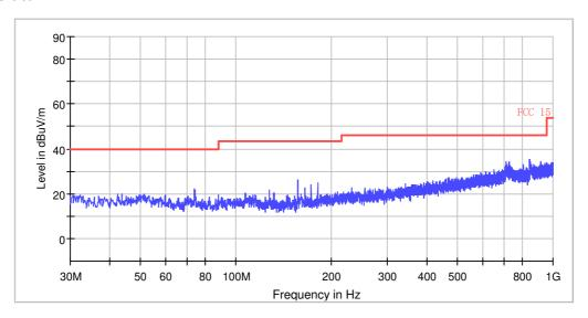
The emission levels with 960 to 1000 MHz also comply with the ICES-005 limit 46 dB $\mu$ V/m.
