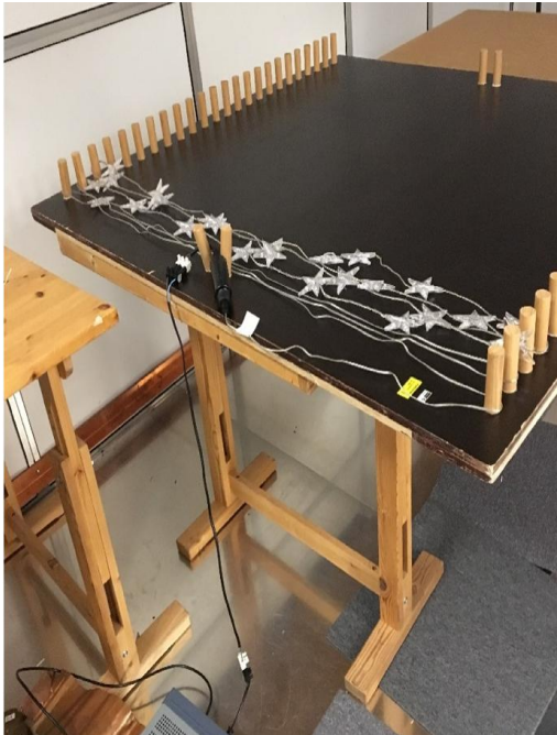
Test setup for conducted emission 150 kHz – 30 MHz
