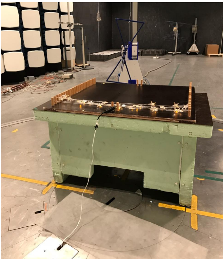
Test set up radiated emission 30 MHz – 1 GHz
