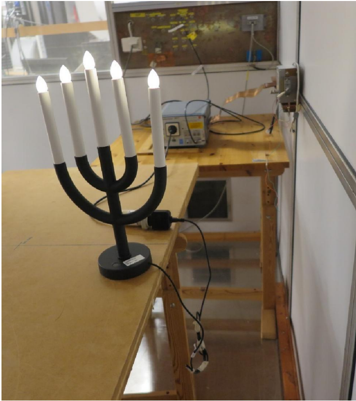
Test setup for conducted emission 150 kHz – 30 MHz
