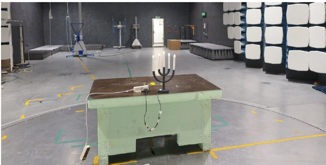
Test set up radiated emission 30 MHz – 1 GHz
