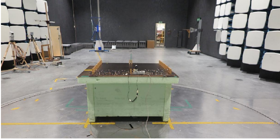
Test set up radiated emission 30 MHz – 1 GHz
