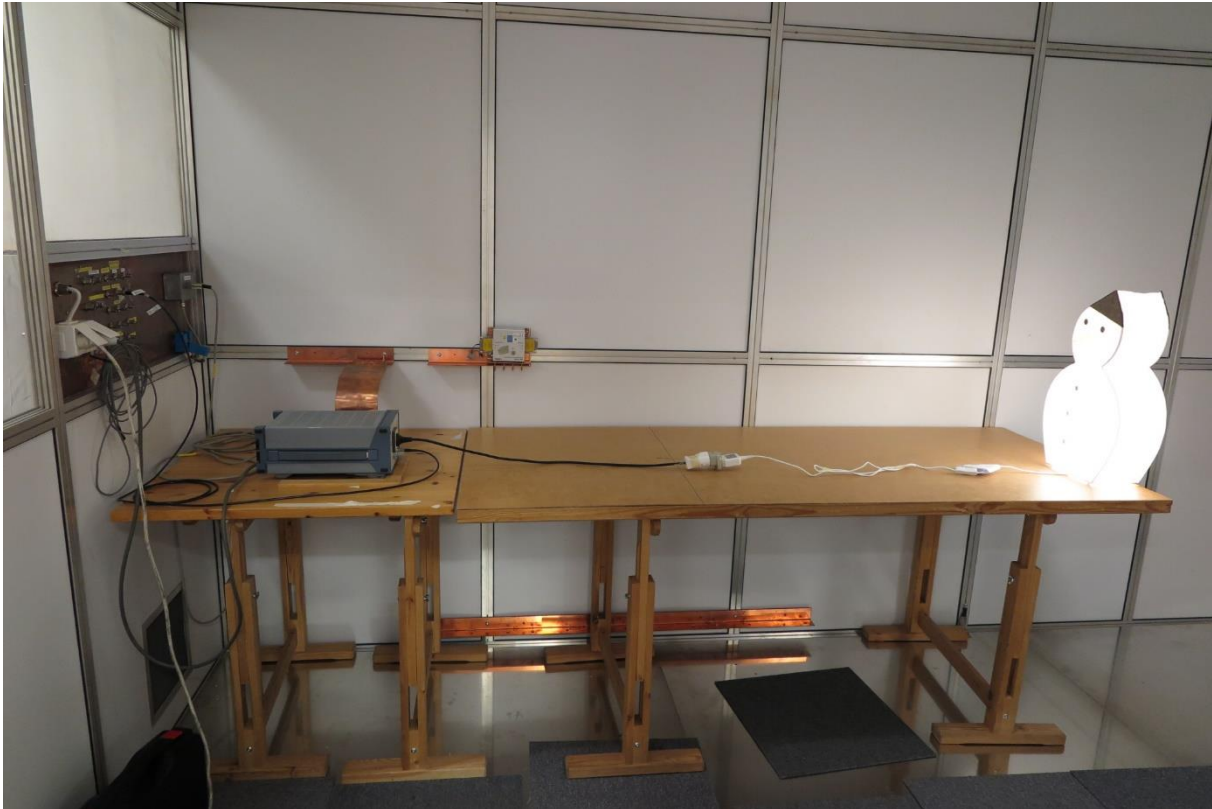
Test setup for conducted emission 150 kHz – 30 MHz
