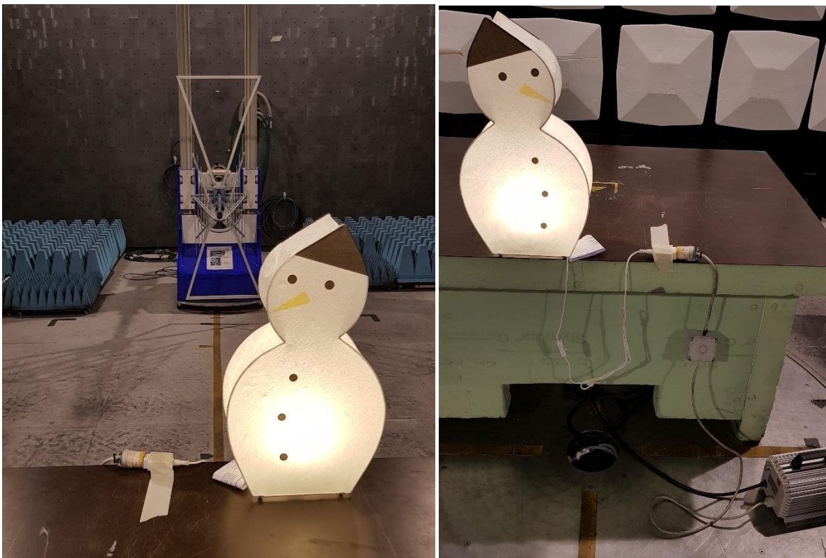
Test set up radiated emission 30 MHz – 1 GHz
