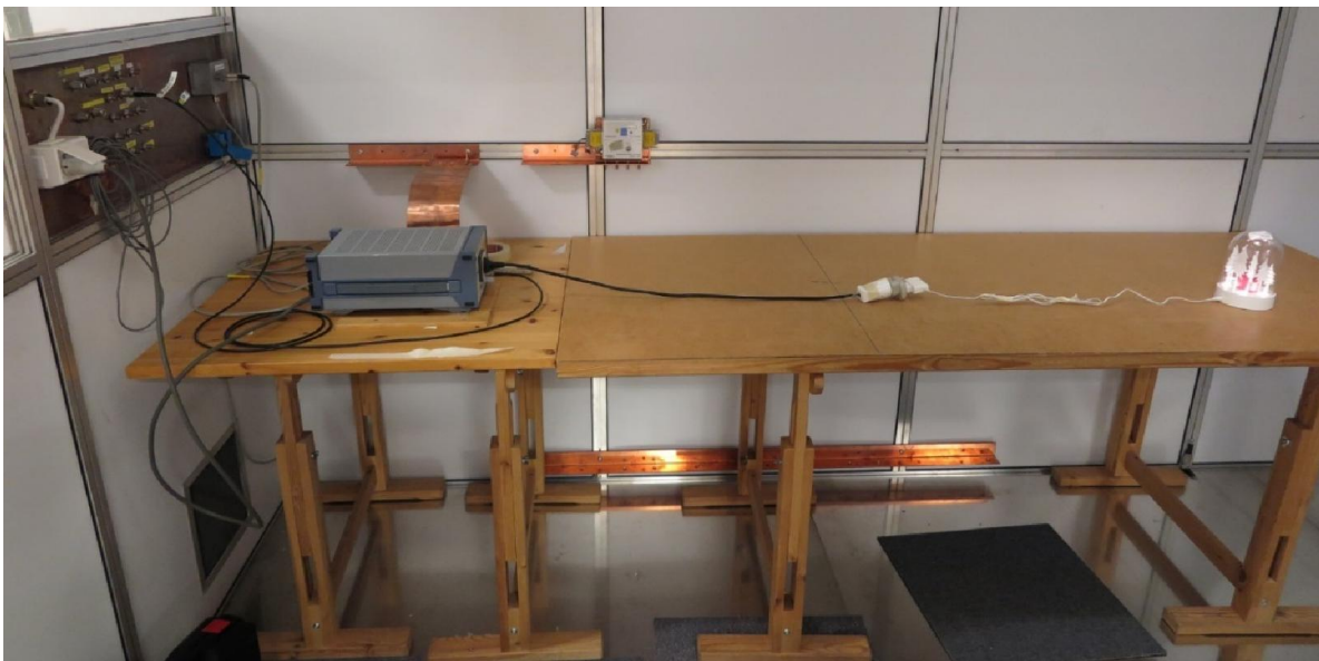
Test set up conducted continuous emission, 0.15-30 MHz
