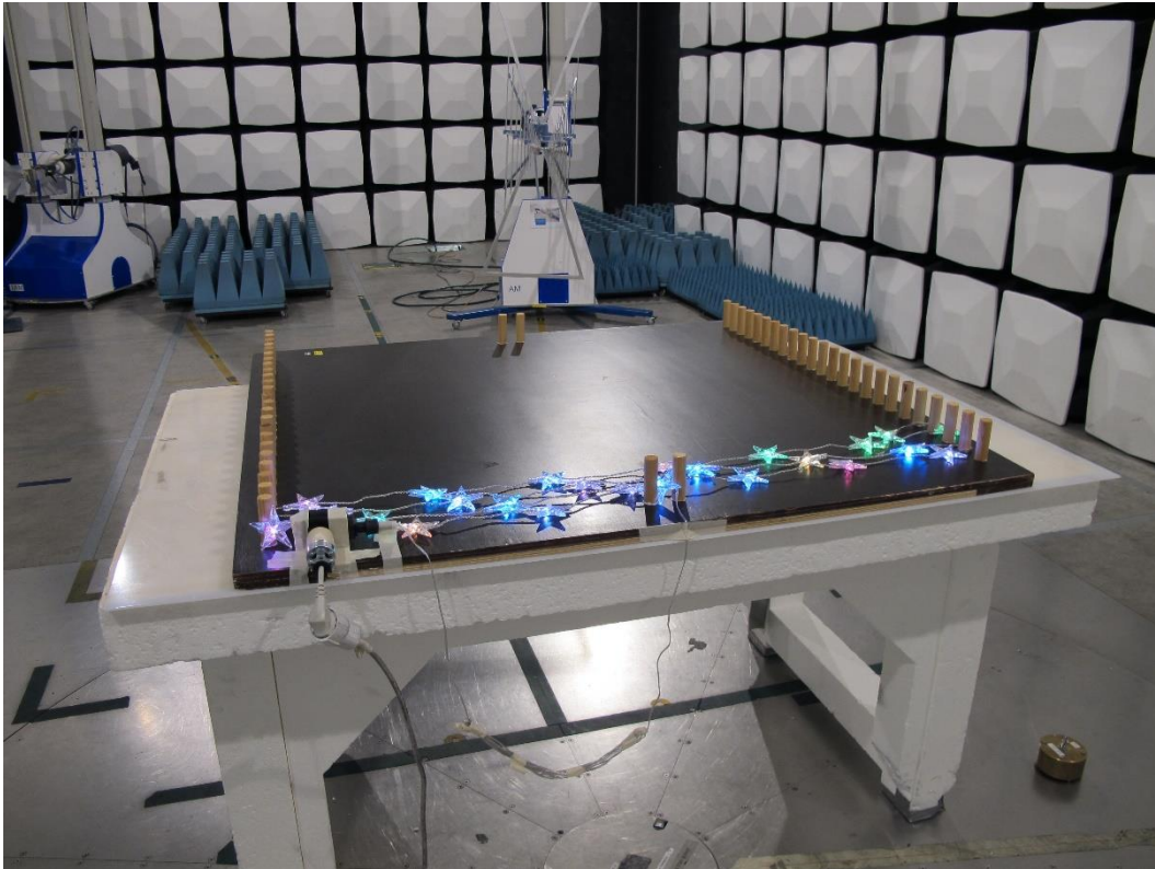
Test set up radiated emission 30 MHz – 1 GHz
