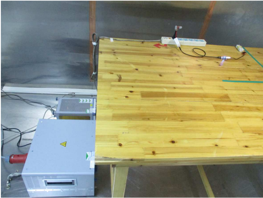
Photograph 2: Set-up for measurement of radiated emission
