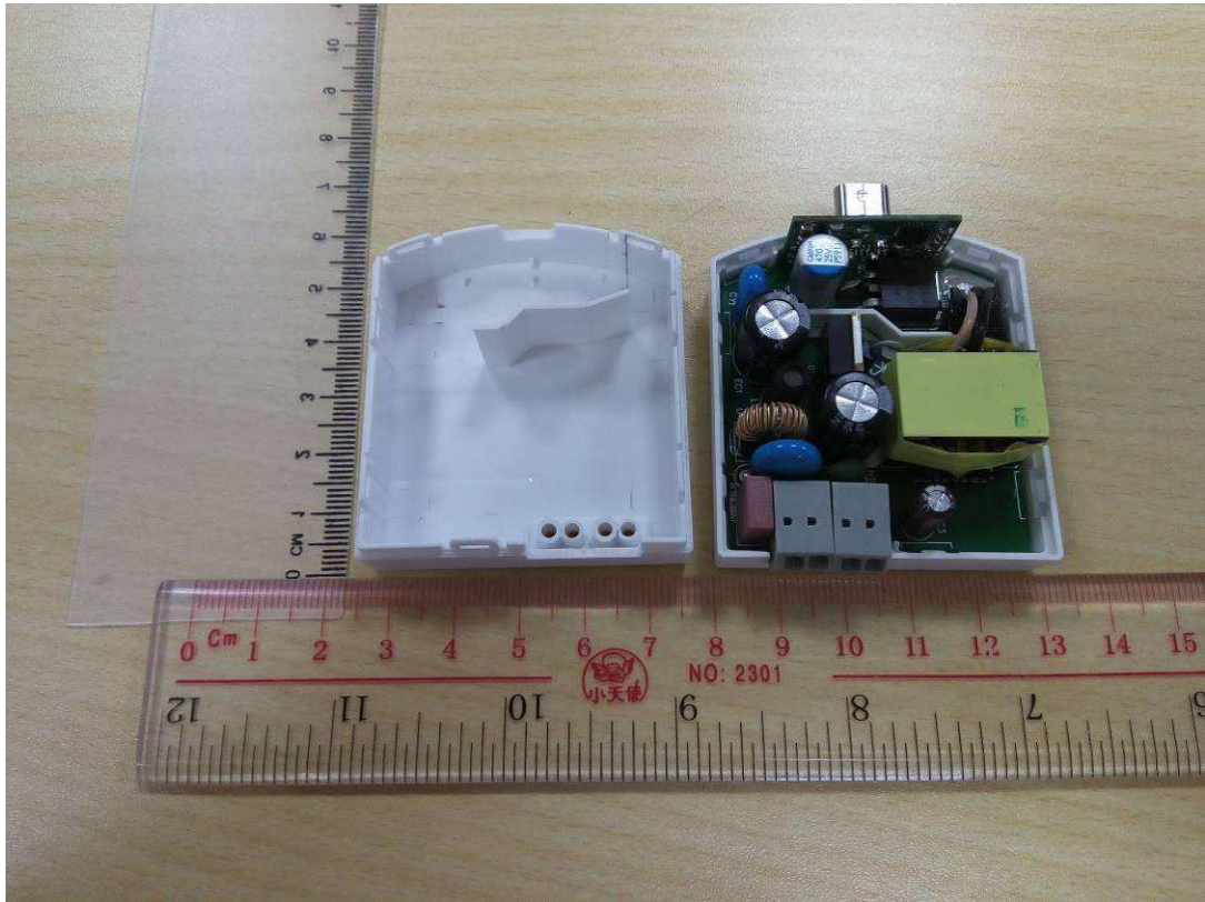
Picture 1 – Internal view (with straight output connector)
