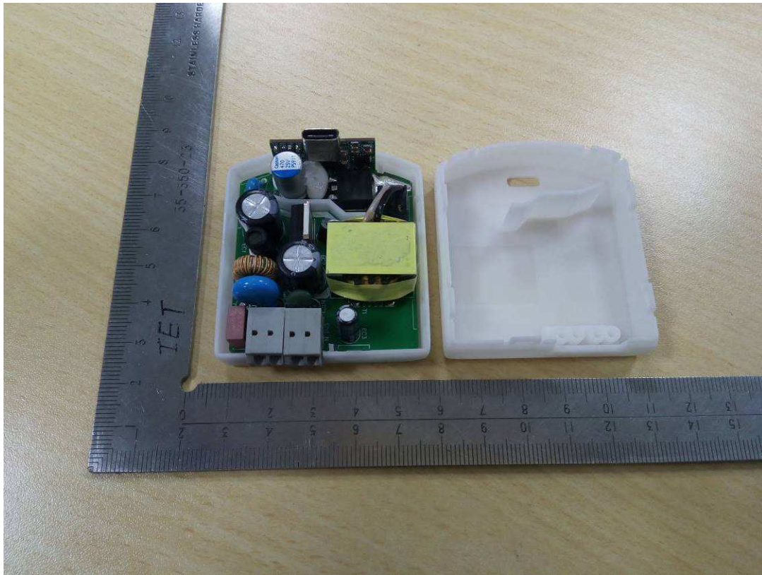
Picture 3 – Internal view (with perpendicular output connector)
