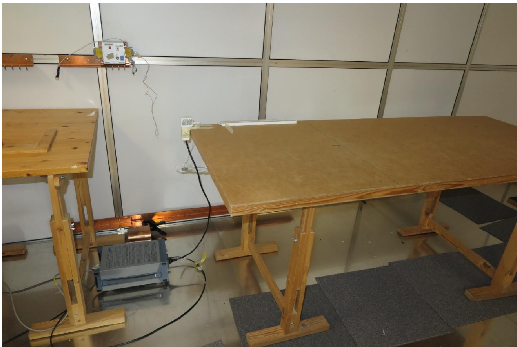
Test setup for conducted emission 150 kHz – 30 MHz
