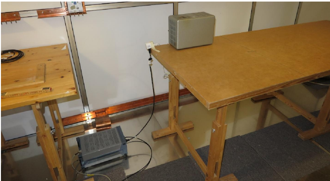
Test set up conducted emission 0.15 MHz – 30 MHz
