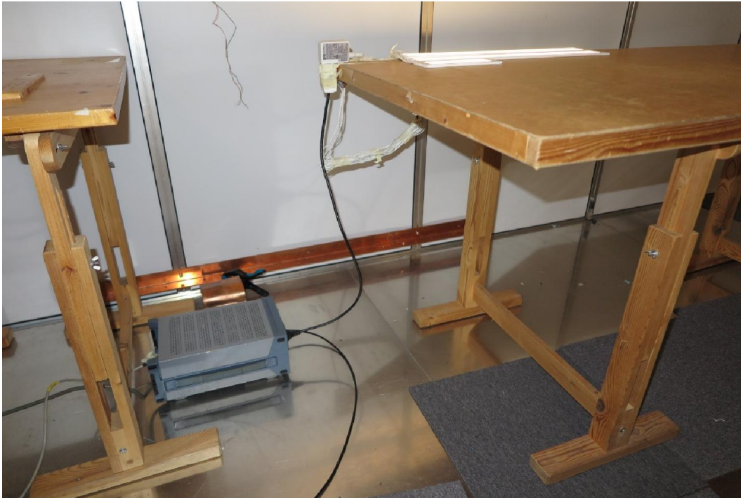
Test setup for conducted emission 150 kHz – 30 MHz, EUT-sample B
