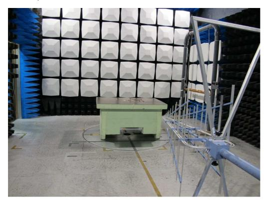
Test set up radiated emission 30 MHz – 1GHz
