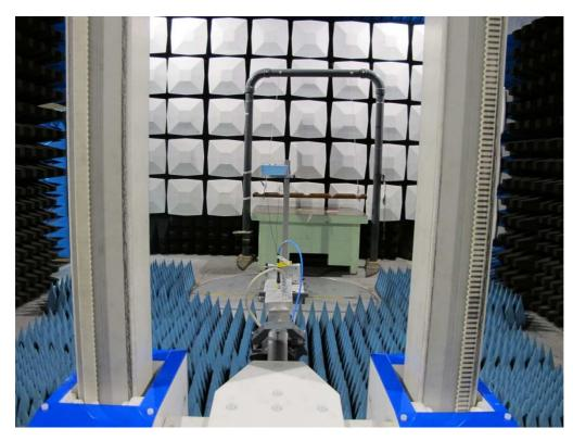
Test set up radiated emission 18 GHz – 26.5 GHz
