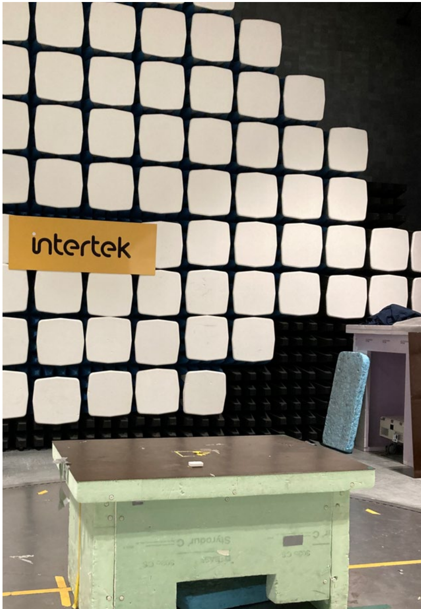
Photo(s) of test setup(s) for radiated disturbances 30 – 1000 MHz
