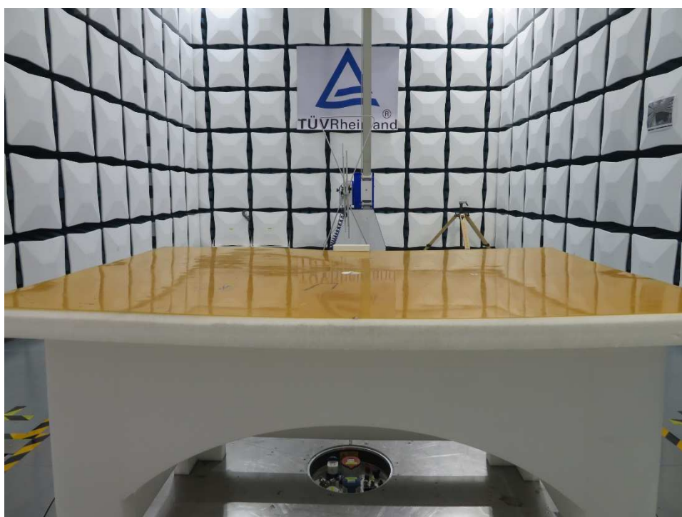
Photograph 2: Set-up photo for Radiated Emission, 30MH - 1GHz
