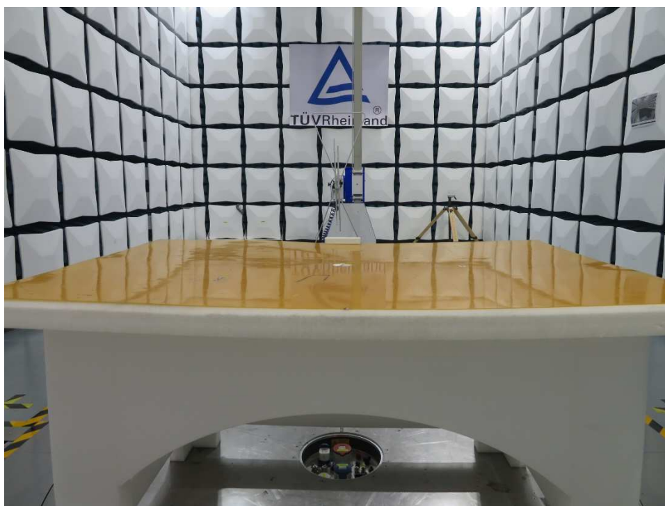
Photograph 1: Set-up photo for Radiated Emission, Below 1GHz
