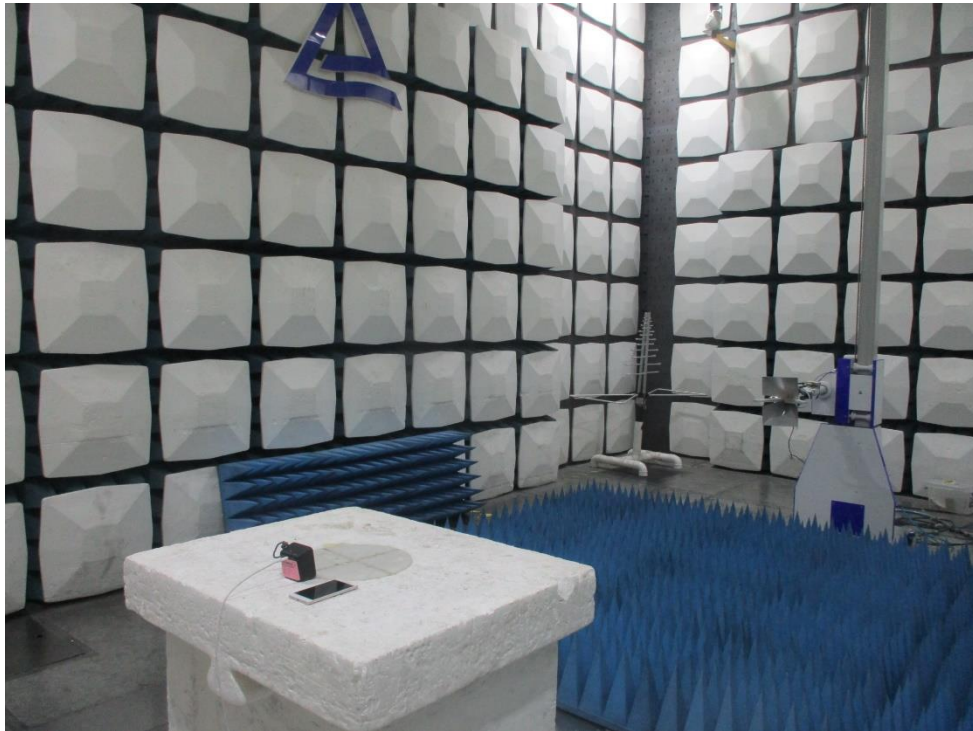
Photograph 3: Set-up photo for Radiated Emission, 1GHz - 18GHz
