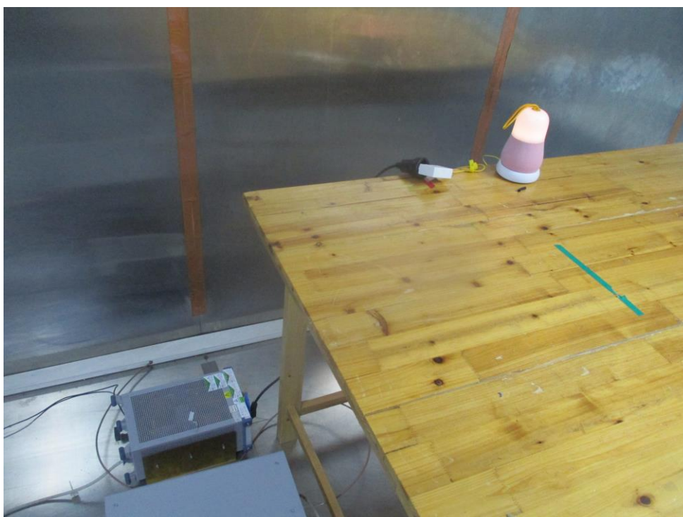
Photograph 2: Set-up photo for Conducted Emission
