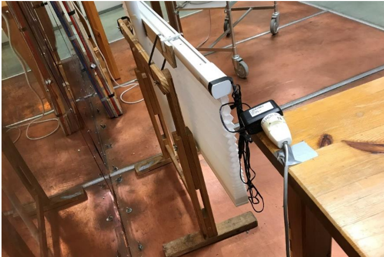
Test setup for conducted emission 150 kHz – 30 MHz
