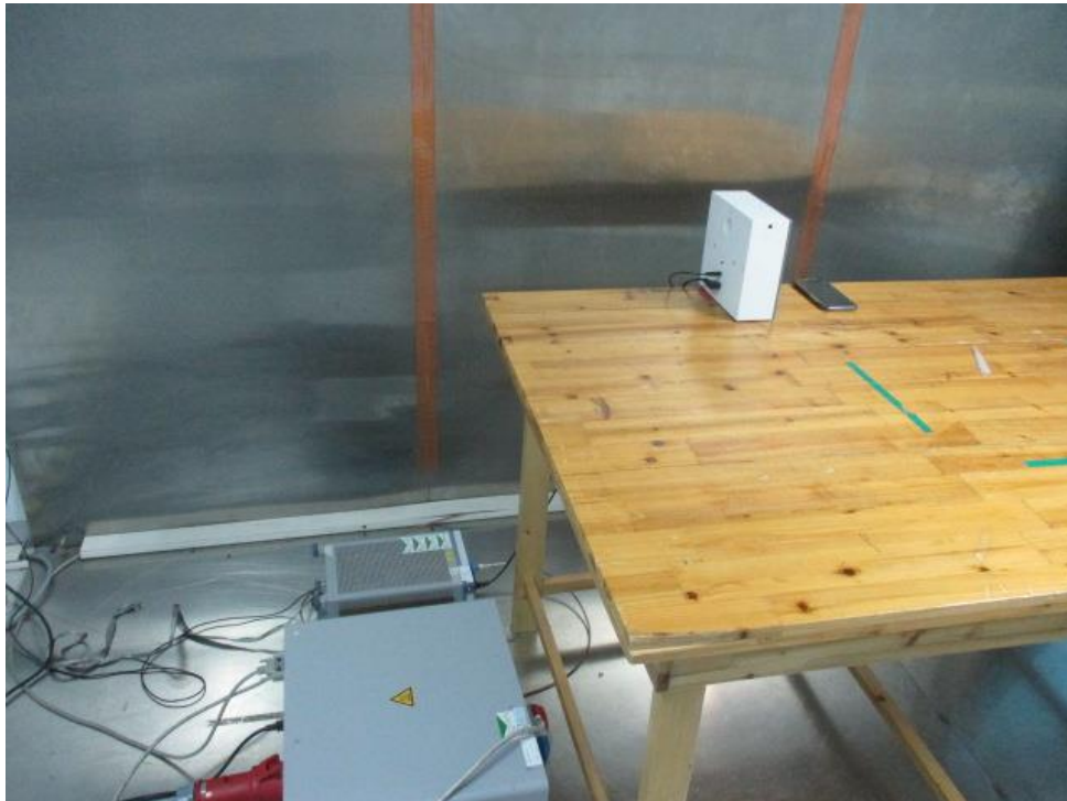
Photograph 2: Set-up photo for Radiated Emission, 30MHz - 1GHz
