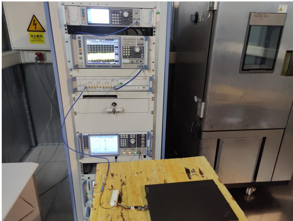
Photograph 1: Set-up photo for RF Conducted Test
