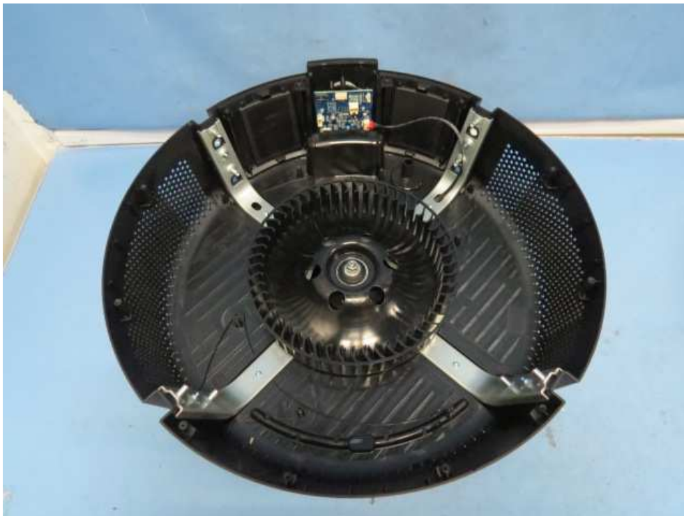
Inner view, location of fan motor
