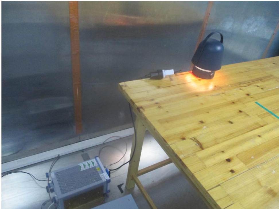
Photograph 1: Set-up photo for Conducted Emission
