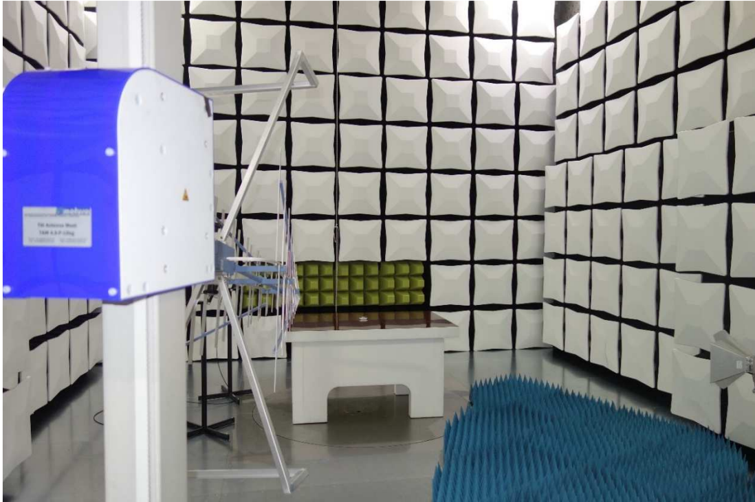
Photo 1: Chamber set up for 30 MHz – 1 GHz
