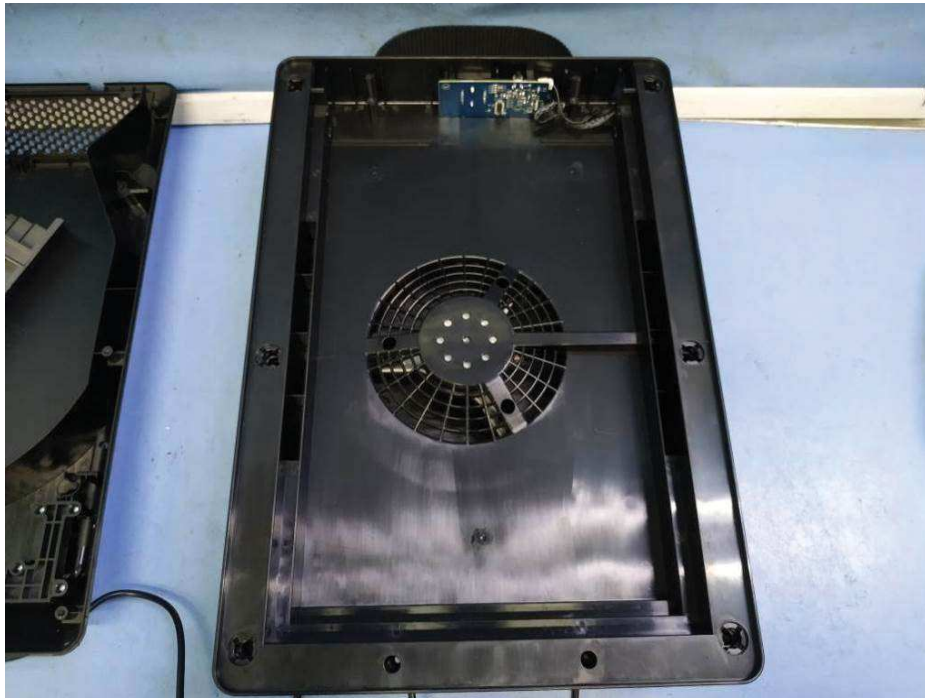
Inner view, location of control board
