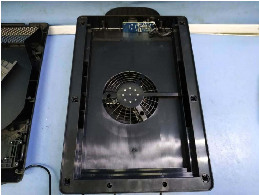
Inner view, location of control board
