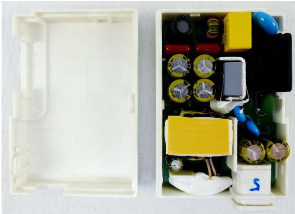
Inner view of adapter (ICPSW24-19-1A)
